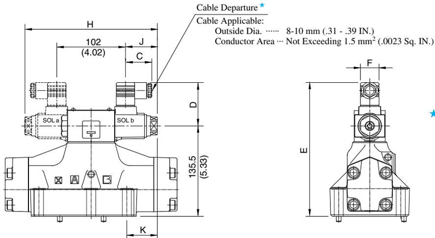
★ Position of cable departure can be changed. For details, refer to DSHG-01 valve on page 396.
